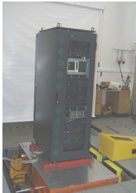
Earthquake test with IT equipment
