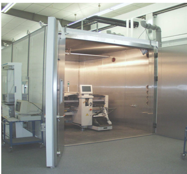
Pick-and-place system undergoing climatic testing
