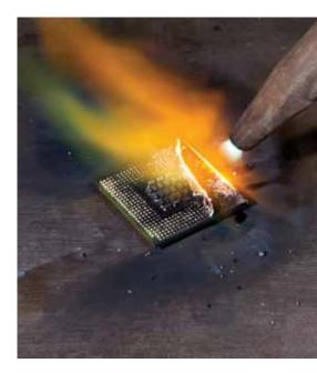
SGS laboratories are qualified to perform burning and flammability tests against the broadest range of international standards and electrical and electronics product categories. See below:
