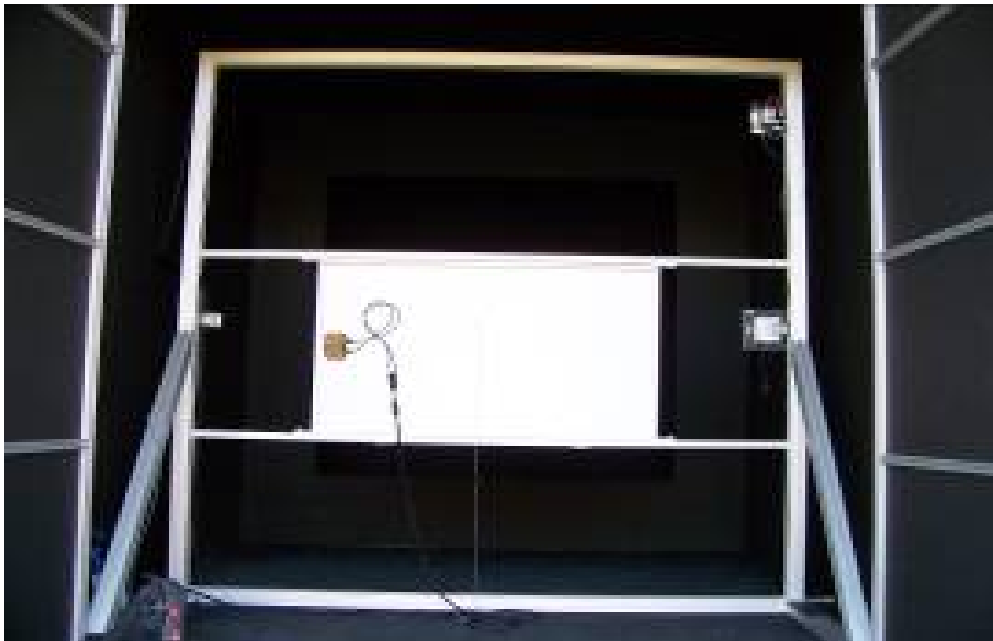
Flasher (Pasan IIIb) Class A/A/A, 3.00m x 3.00m → Leistungsbestimmung
