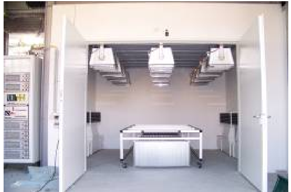
UV chamber 2.40m x 2.80m → UV-Schädigung
