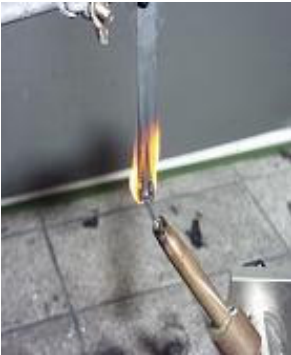
Ignition of a test bar according UL 94
