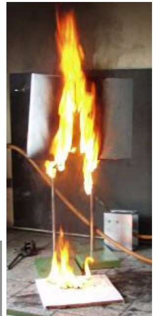
Flammability test on enclosure according EN 60950 Annex A.1
